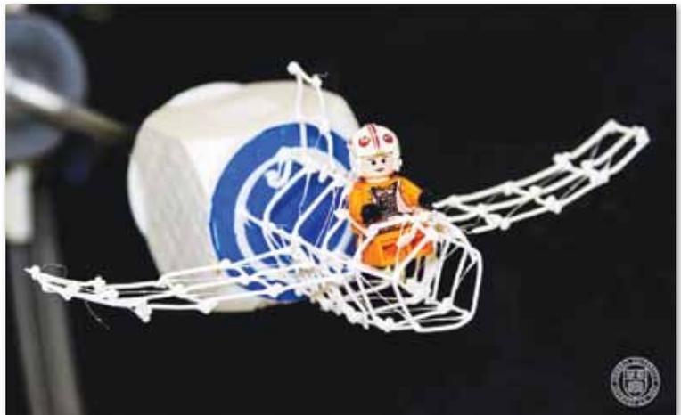
*A wire frame prototype of a toy aircraft for a Lego kit was printed in just 10 minutes, including testing for correct fit.*
